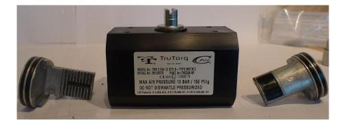
A6. Remove the pistons out of the body by turning the top of the shaft, anti-clockwise\*, by using an appropriate tool.
