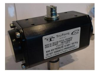
A1. Check/note the shaft position, when the actuator is in a unpressurised state, in relation to the actuator before the dismantling. The intention is to ensure that the actuator has the same function after reassembly (Fail Closed, Fail Open or Crossmount).
