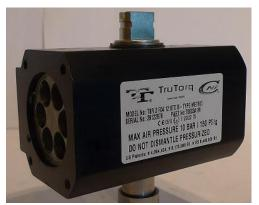
A5. Check/note the position of the pistons before you take these out of the actuator. The intention is to ensure that the actuator has the same function after reassembly.
