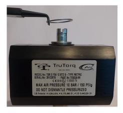
A7. Remove the Circlip at the top of the driveshaft by using external drop nose Circlip pliers. Then remove the washer.
